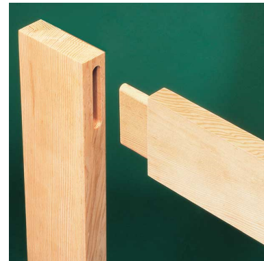
Example of Socket (joint) and Tenon
